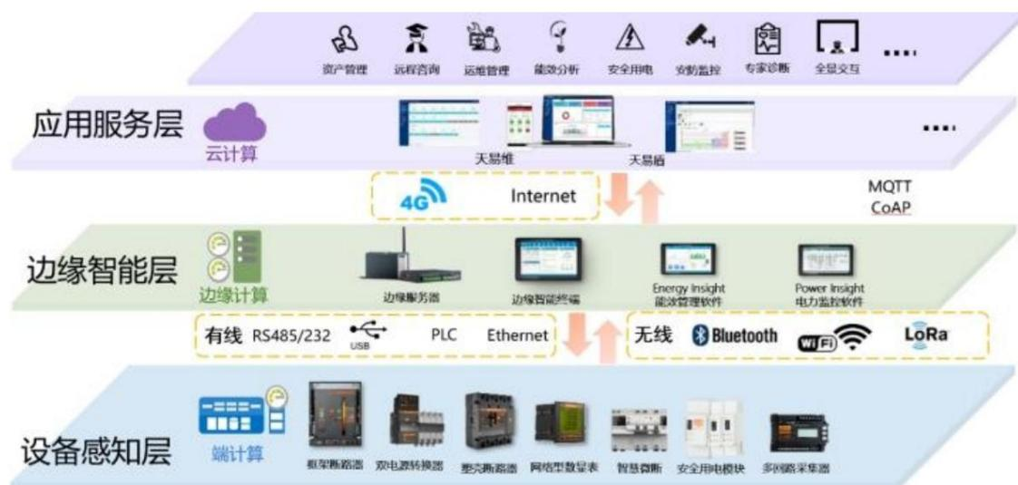
The company's Tianzheng Tianzhi "TenEdge" intelligent power distribution system is based on the Internet of Things architecture, relying on built-in intelligent circuit breakers, modules, etc.
